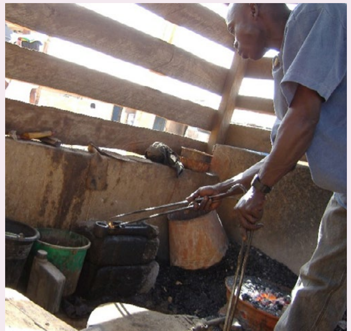
Plate 1: Miners burning mercury amalgam without protective equipment is a common sight.
