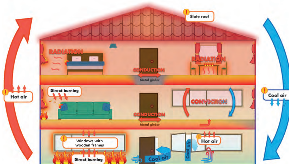
Figure 3: How types of heat transfer contribute to fire spread
